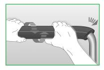
Push the Armaflex along the pipe using a circular motion. **Do not pull the insulation.**
