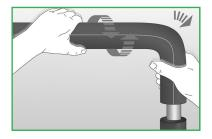
Using a circular motion, push the Armaflex around bends. **Do not pull the insulation.**
