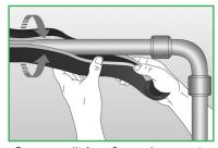
Open pre-slit Armaflex and snap onto pipe (the release paper is still protecting the self-adhesive strip)
