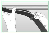
Adjust fitted Armaflex to ensure slit is easily accessible.
