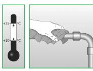
Clean all dust, dirt, oil and water from pipework using Armaflex cleaner where necessary. Install Armaflex when ambient temperature is between +10 and +35°C.
