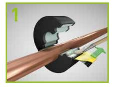
Install Armafix Ecolight pipe support on the pipe, seal the surfaces using Armaflex adhesive and remove the protective paper strip on the overlapping PVC cover.
