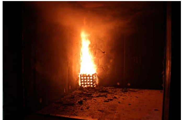
Figure 4: FM 4924 room test.
