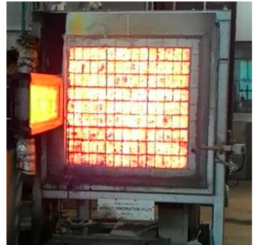
Figure 1: Test chamber for BS476 Part 7 fire test.
