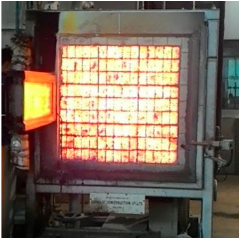
Figure 1: Test chamber for BS476 Part 7 fire test.
