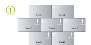
Work out the most efficient way of covering the surfaces using ArmaFlex Pro. Ensure that sheet joints are staggered. Cut ArmaFlex Pro insulation sheets to size, including 5 mm of additional allowance on all sides to enable compression joints.
