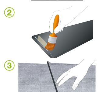
Leaving a gap of about 30 mm from the edge, apply a thin and even coat of ArmaFlex 520 adhesive onto both surfaces to be glued. When adhering ArmaFlex Pro to other materials (e.g. metal), apply adhesive to the insulation material first, then on the other clean surface.
