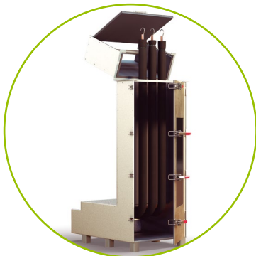
Insulated pipes are first inserted into a vertical pipe chase test chamber which mimics the actual pipe installation.
