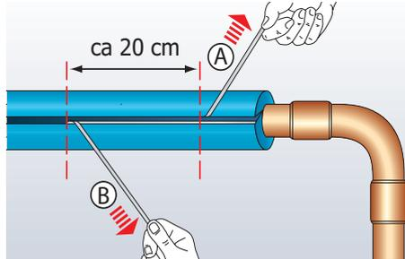
Remove the white protection paper strip on both sides, by drawing it away from the insulation. Please note: remove protective release paper strip from both sides!
