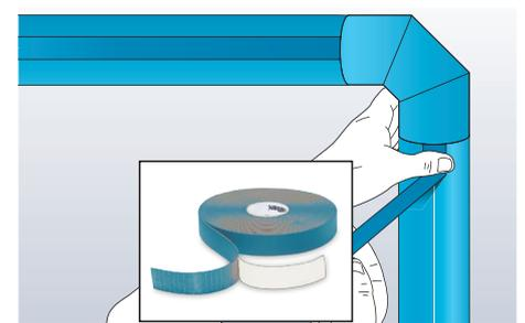
For additional security it is necessary to secure the longitudinal joints of Armaflex Ultima self-adhesive tubes with an additional Armaflex Ultima self-adhesive tape. Ensure that the surface is clean, dry and free from contamination, if necessary please clean it with Armaflex cleaner.
