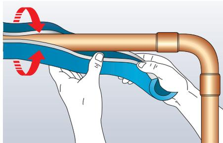
Open pre-slit Armaflex Ultima and snap onto pipe (the release paper is still protecting the self-adhesive strip).
