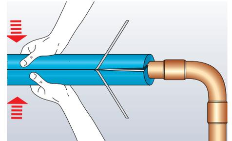
Close the slit seam and press together firmly to ensure a permanent seal.
