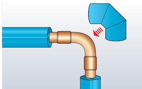
Insulate all other straight pipe sections following the previous described procedure. Finally insulate all elbows, T-pieces etc. following Armaflex Application Manual instructions.
