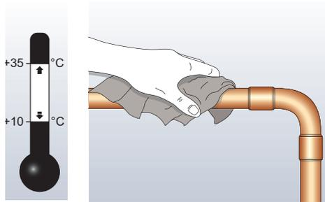
Clean all dust, dirt, oil and water from pipe-work using Armaflex cleaner where necessary. Install Armaflex Ultima self-adhesive when ambient temperature is between +10 and +35 °C.
