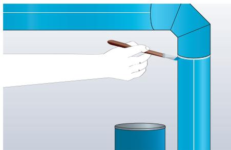
Seal all joints with Armaflex adhesive. Do not stretch when sealing joints. When gluing joints under compression, with no gaps present, the wet adhesive method should be applied.
