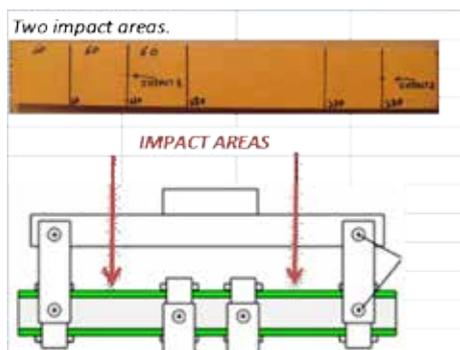
in the core when testing in 4-point bending mode, see fig. 3. The beams were tested for two different boundary conditions. At first the beams were fully supported on the back side when impacted, resting on a stiff aluminum profile.
