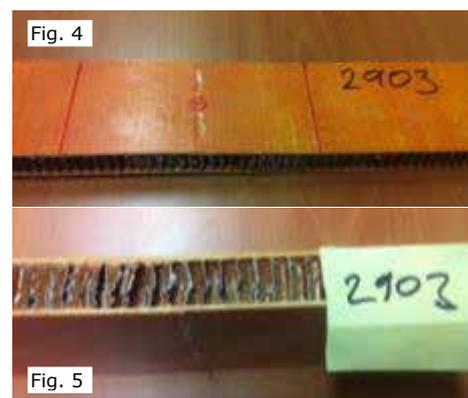
is marked. Note the **permanent deformation and damage to the skin**. Figure 5 shows typical **buckling damage** to the honeycomb core cell walls under the impact location.
