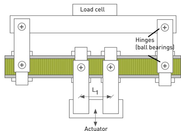
Figure 1: Four-point bending test setup
