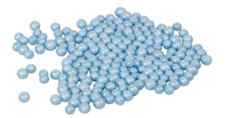
Cement and concrete are important materials for building and construction purposes. Adding ArmaShape as a filler substitution generates a better strength to weight ratio, allowing for improved lightweight construction and positively impacting the sustainability of the solution.
