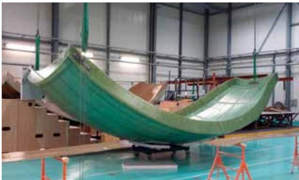
©Multiplast: panels cored with ArmaForm GR80 in 50 mm
