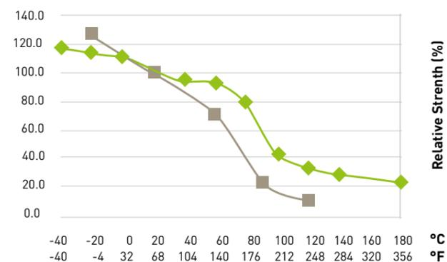
Figure 2: Relative compressive strength vs. temperature.
