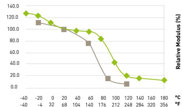
Figure 1: Relative compression modulus vs. temperature.
