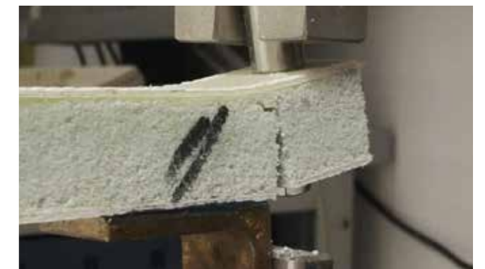
Figure 4: Peel off test on a sample
