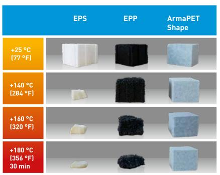
Moulded ArmaPET Shape H has an excellent thermal stability for further processing at elevated temperatures, such as infusion and RTM. It is extremely tolerant to high-peak exothermic reactions and shows no degradation of material properties even in the case of hot spots.
