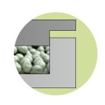
The mould should be designed in such a way that the top part allows the compression of the beads inside the mould. Therefore, the upper part of the mould needs to fit into the bottom part as shown in the illustration. The top part can also be designed with a ribbing structure that ensures the required compression and would leave a pattern on the final part.
