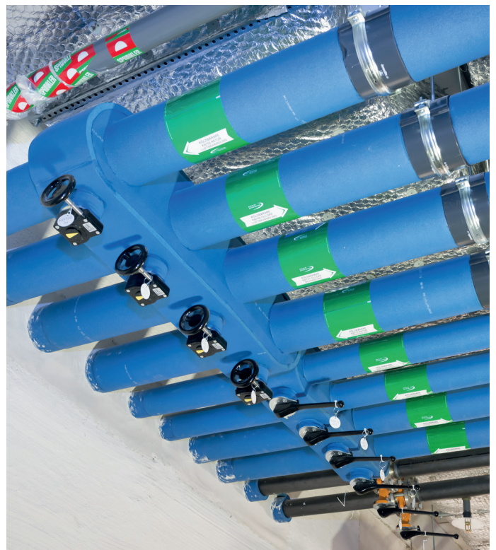
Armaflex Ultima pipe supports ensure that the pipe is isolated from the bracket and thus prevent thermal bridges
