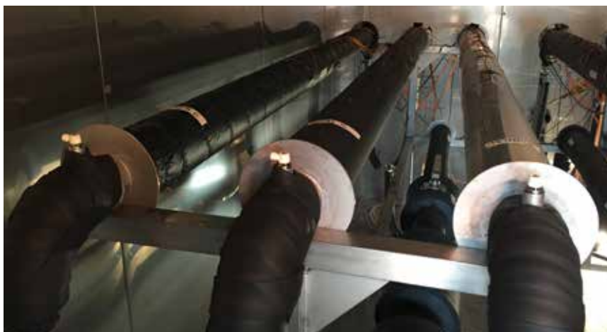
Figure 3: Test set-up: The test specimens in the climate chamber
