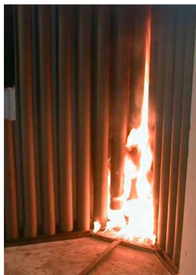
Figure 2: The SBI test – shown here with elastomeric tubes – before, during and after the test
