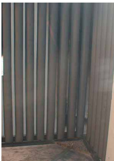
Figure 2: The SBI test – shown here with elastomeric tubes – before, during and after the test
