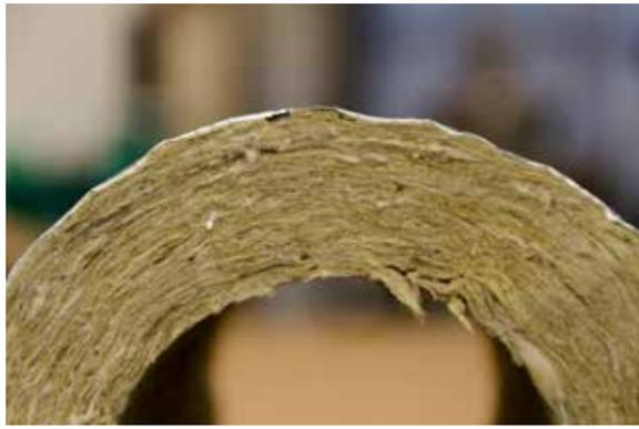
Because it is an open-cell insulation material, mineral wool is not protected against moisture penetration and, therefore, should not be installed on refrigeration pipes.
