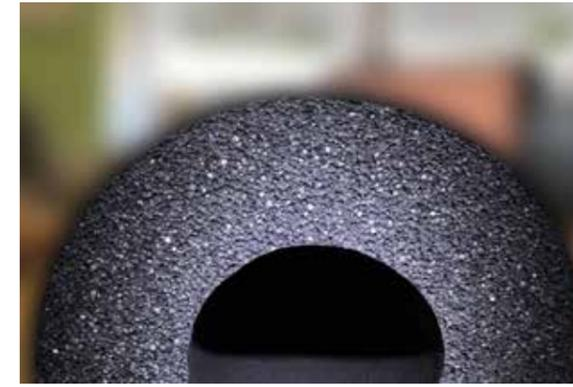
Elastomeric insulation materials have a closed-cell structure and a high resistance to water-vapour transmission, so they do not need a separate vapour barrier and can be installed easily, quickly and reliably.
