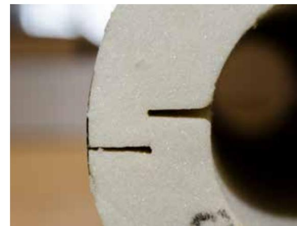
Rigid PUR/PIR foam has a low resistance to water-vapour transmission and therefore needs an effective vapour barrier
