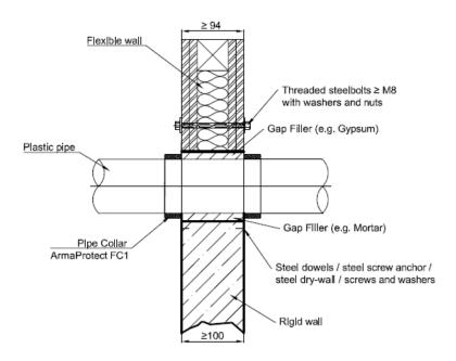
Penetration of pipes, floor installation - section view Penetration of pipes, floor installation - section view
