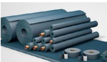
Thanks to its good thermal conductivity and high resistance to water vapour diffusion, the low-smoke ArmaFlex Ultima ensures reliable condensation control and high energy savings in the long term. This also minimises the risk of corrosion under insulation (CUI) and reduces the risk of costs associated with downtime. It can be used on cold service pipework for refrigeration systems everywhere onboard.
