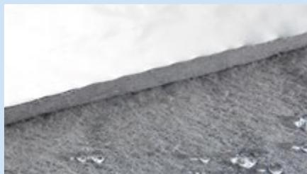
Thanks to its exceptionally low thermal conductivity, ArmaGel is one of the best insulation materials available today. It is up to 80 percent thinner than conventional insulation and offers the same thermal insulation properties with only a fraction of the insulation thickness.
