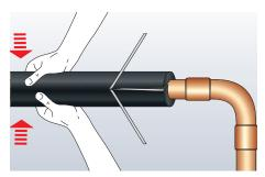
Close the slit seam and press together firmly to ensure a permanent seal.
