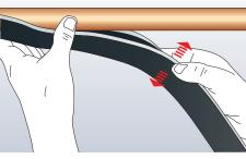
Adjust fitted NH/Armaflex to ensure slit is easily accessible.
