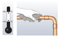
Clean all dust, dirt, oil and water from pipe-work using Armaflex cleaner where necessary. Install NH/Armaflex self-adhesive when ambient temperature is between +10 and +35 °C.
