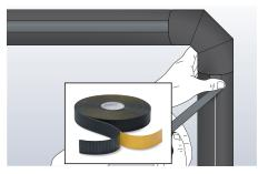
For additional security it is necessary to secure the longitudinal joints of NH/Armaflex self-adhesive tubes with an additional **NH/Armaflex self-adhesive tape**. Ensure that the surface is clean, dry and free from contamination, if necessary please clean it with Armaflex cleaner.
