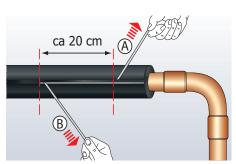
Remove the white protection paper strip on both sides, by drawing it away from the insulation. Please note: remove protective release paper strip from both sides!
