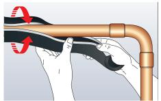
Open pre-slit NH/Armaflex and snap onto pipe (the release paper is still protecting the self-adhesive strip).
