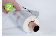
Press the longitudinal join together, peel off the protective strip of the closure and press the adhesive tape down firmly. The surfaces to be bonded must be dry and free of dust or grease.
