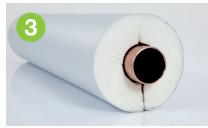
To minimise heat losses, when installing horizontally ensure that the longitudinal seam is located on the underside of the pipe (at 6 o'clock).\* Secure the butt joints of the pipe shell with suitable adhesive tape.
