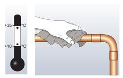
Clean all dust, dirt, oil and water from pipe-work using Armaflex cleaner where necessary. Install Armaflex Ultima self-adhesive when ambient temperature is between +10 and +35 °C.
