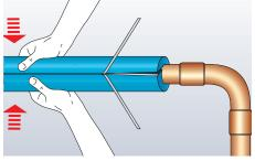
Close the slit seam and press together firmly to ensure a permanent seal.
