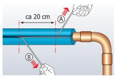
Remove the white protection paper strip on both sides, by drawing it away from the insulation. Please note: remove protective release paper strip from both sides!
