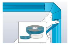
For additional security it is necessary to secure the longitudinal joints of Armaflex Ultima self-adhesive tubes with an additional Armaflex Ultima self-adhesive tape. Ensure that the surface is clean, dry and free from contamination, if necessary please clean it with Armaflex cleaner.
