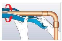
Open pre-slit Armaflex Ultima and snap onto pipe (the release paper is still protecting the self-adhesive strip).
