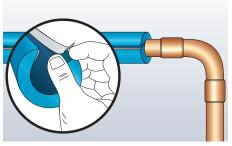
Locate the end of white release paper for the self-seal strip.
