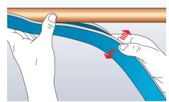
Adjust fitted Armaflex Ultima to ensure slit is easily accessible.
