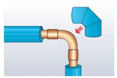
Insulate all other straight pipe sections following the previous described procedure. Finally insulate all elbows, T-pieces etc. following Armaflex Application Manual instructions.
