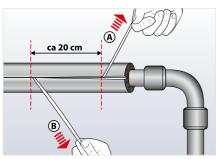
2. Remove the protection paper strip on both sides, by drawing it away from the insulation.
