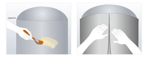
2. Transfer the circumference to the Arma-Chek Silver sheet and cut to the required size. Spread a thin film of adhesive onto the Arma-Chek Silver sheet and then onto the metal surface. When the adhesive is tack dry (fingernail test) place Arma-Chek Silver sheet in position and press firmly to achieve a good bond. Fix the first Arma-Chek Silver sheet to the height of the tangent line.
