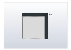
Especially on the corners of the flange, but also on all corners of the air-duct system, the Arma-Chek factory-covered sheets and strips can be cut with a  $45^{\circ}$  angle.
