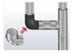
The correct size of the prefabricated covers for insulated pipe bends depends on the pipe diameter and insulation thickness. Consult the following table to select the correct prefabricated cover.
