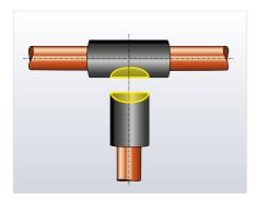
Cut a hole in the non-covered Armaflex tube for the main pipe with a sharpened section of copper pipe of the correct diameter.
