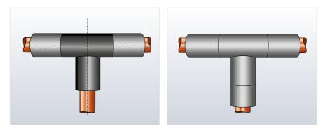
Afterwards install the T-piece section, gluing it onto the pipe and cover this area with the prefabricated Arma-Chek Silver T-piece.
