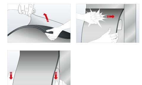
Peel back 10 to 20 cm of the protective foil and position the sheet.
