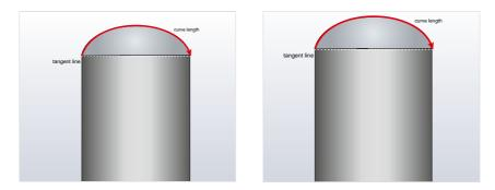
1. Determine the curve length (a) of the insulated vessel dome end using a tape measure.
