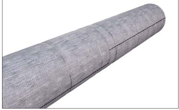
Figure 12: Rotate longitudinal seams to side
