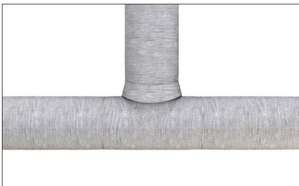
Figure 51: Installation of tee cover.
