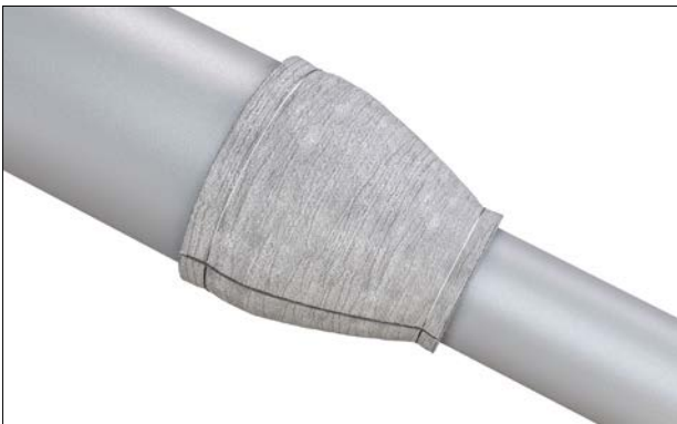
Figure 47: Securement of reducer.
