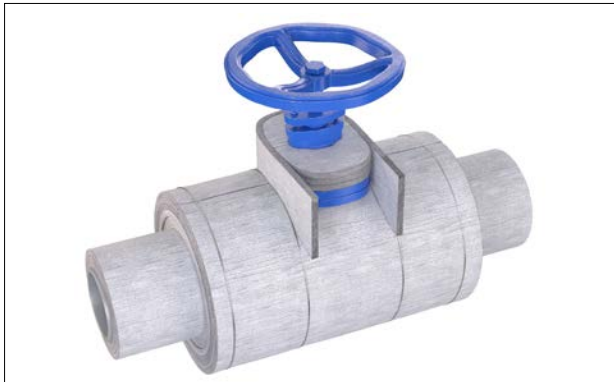
Figure 62: Fabricate spindle bonnet cap.
