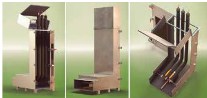
Figure 4: NFPA 274 test apparatus.
